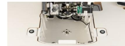
The wiring inside and outside the machine head is neatly tucked away under the machine head for easy cleaning.
