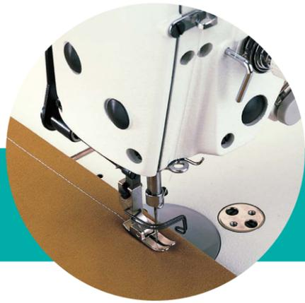
It has inherited the advanced features of the DDL-9000 Series, such as the direct-drive system, semi-long arm and elimination of the oil pan. In addition, it comes with a highly reliable needle feed mechanism.
